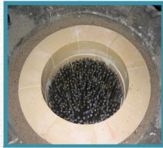
▲ Melt trap before and after RT-11 experiment (CORMIT-2)
