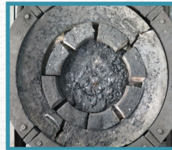
▲ Melt trap before and after RT-11 experiment (CORMIT-2)
